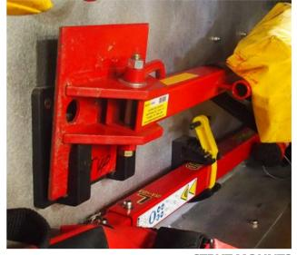
STRUT MOUNTS Vertical Mount & Horizontal Mount Part #: JYD-1090K
