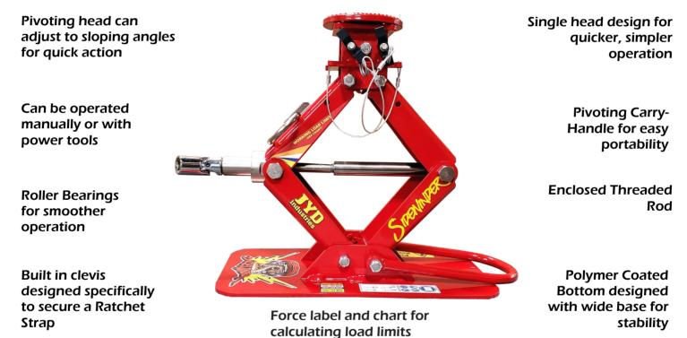
The SIDEWINDER is designed for rescue operation to either stabilize or lift an intended load. A choice of heads gives a choice of smooth or aggressive action against the load. Pivot head provides better surface contact on angled loads. The smooth operating drive train provides ease of operation - manually or by a powered impact tool. In operation, the SIDEWINDER increases in strength as it is extended.
